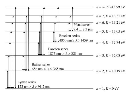
**Fig. 1.2** Energy level diagram and spectral series of the H atom. The levels corresponding to the principal quantum numbers  $7 < n < \infty$ have been left out. The energies given are relative to the ground level n = 1. The ionization energy corresponds to  $n = \infty$ . It should be noted that the distances between the energy levels is not shown to scale.
