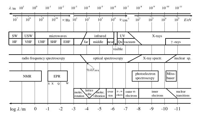
Fig. 1.3 Spectroscopy and electromagnetic spectrum over 14 orders of magnitude of the wave length.
